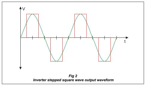
This is important for circuits where magnetic devices, such as transformers and contactors (RMS voltage) are in circuit with electronic relays that derive their DC voltage from capacitor input filters (peak voltage).
